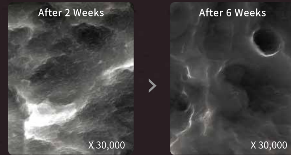
Coating layer is present Coating layer is absorbed
